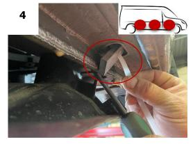
Insert the HTCOR3 into the area marked in the figure.
