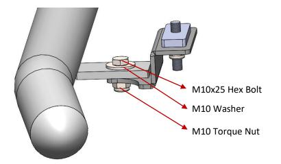
Place sidebar to the brackets ( bolds) and tighten them with nuts and rivets.
