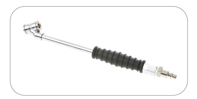
Designed for applications where a long reach chuck is required such as Bead locks, split rims and dual truck rims, this push on air chuck can be fitted to ARB compressor lines with the US standard fitting, or the fitting can be removed and retrofitted with any air fitting using ½ NPT thread
